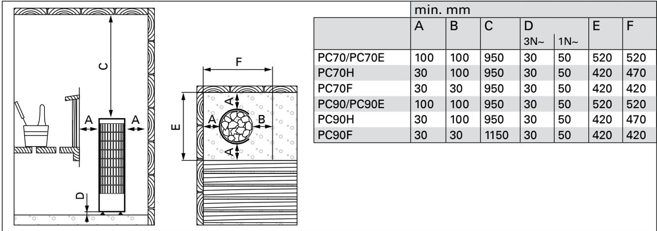
Figure 6. Safety distances (all dimensions in millimeters)
