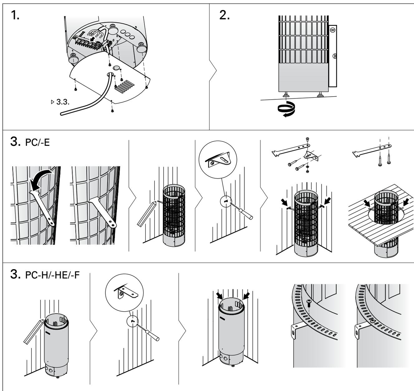
Figure 9. Installing the heater
