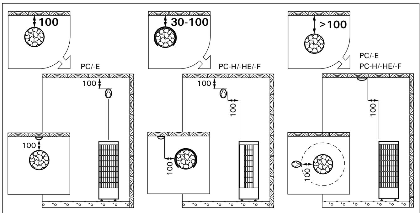
**Figure 8. Installing the sensor (all dimensions in millimeters)**
