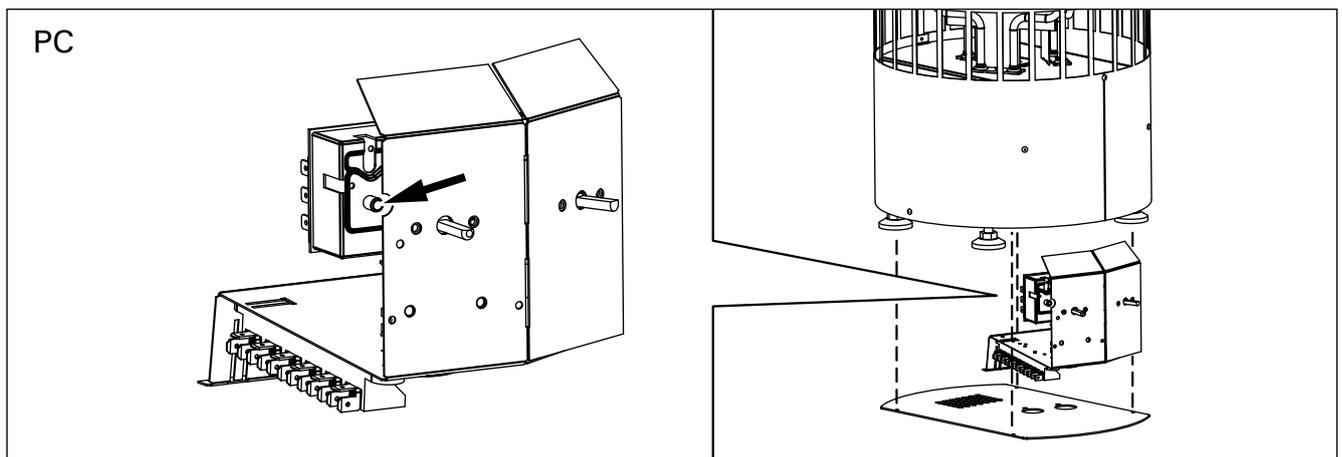
Figure 10. Reset button for overheat protector
